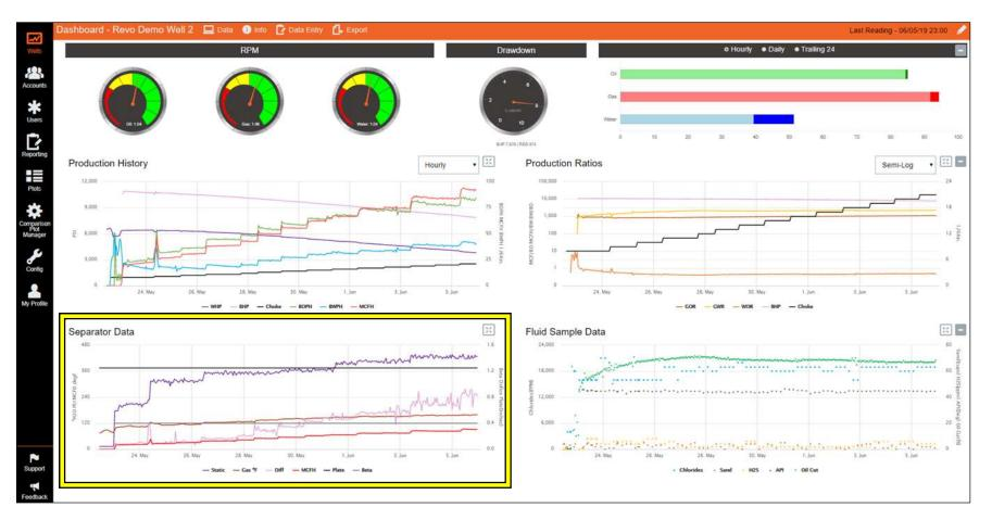
• The separator data plot in the lower left of the dashboard is used to monitor separator data trends and trouble shoot gas rate measurement errors
