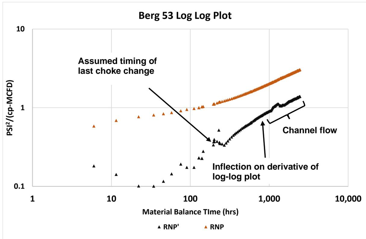
Figure 18 - Log-log plot of initial production (first 22 days) data for Berg 53H
