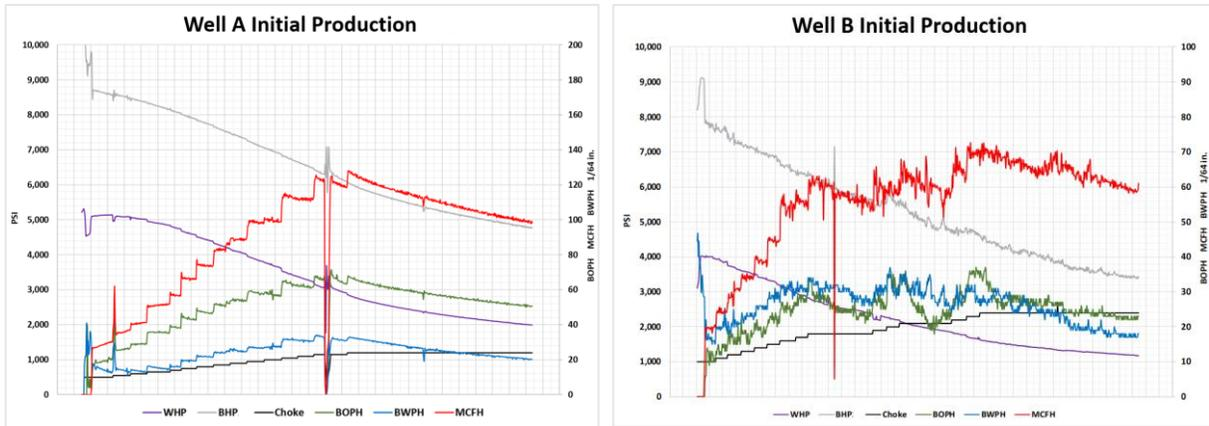
Figure 6 - Initial Production (flowback) History Plot with engineered flowback and superior data quality (Well A) and poor data quality (Well B)
