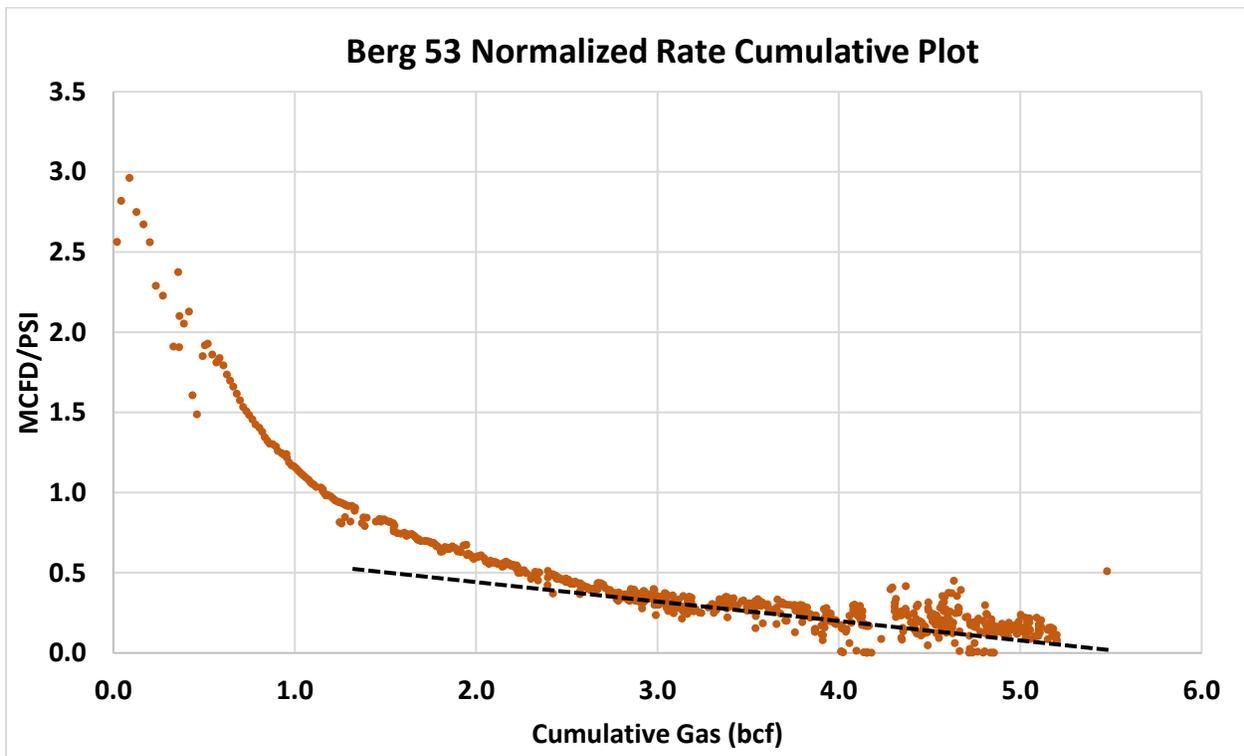
Figure 22 – Normalized Rate Cumulative plot with 6 years of data indicating total contacted volume at 6 years
