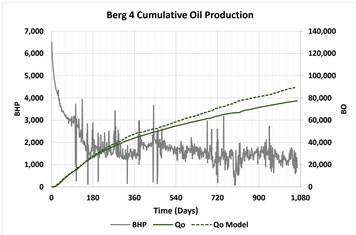
Figure 29 - Cumulative oil comparison between data and model for Berg 4 with no adjustments for boundary effects
