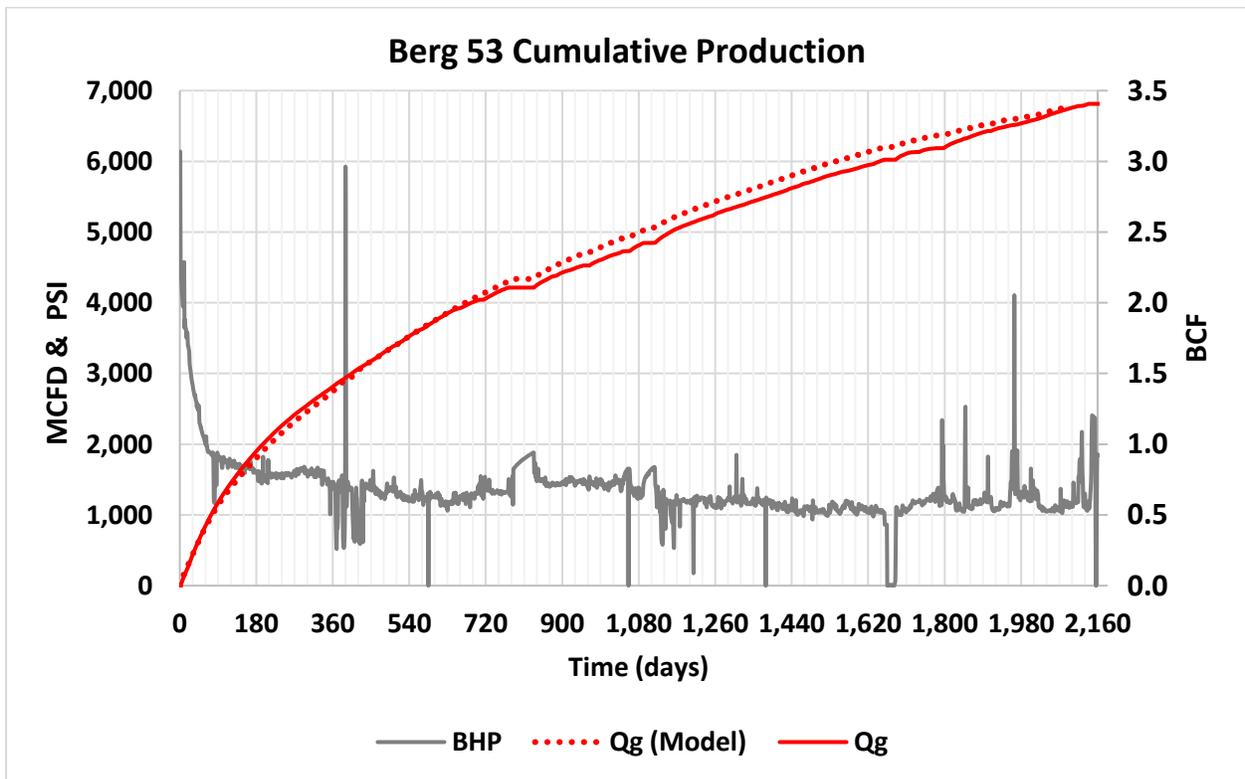
Figure 24 - Production History showing model match constrained with the contacted volume in Figure 20
