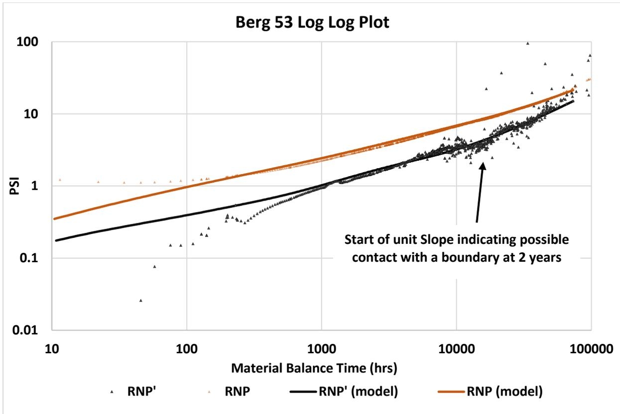
Figure 23 - Log-Log Plot indicating a unit slope starting at 2 years
