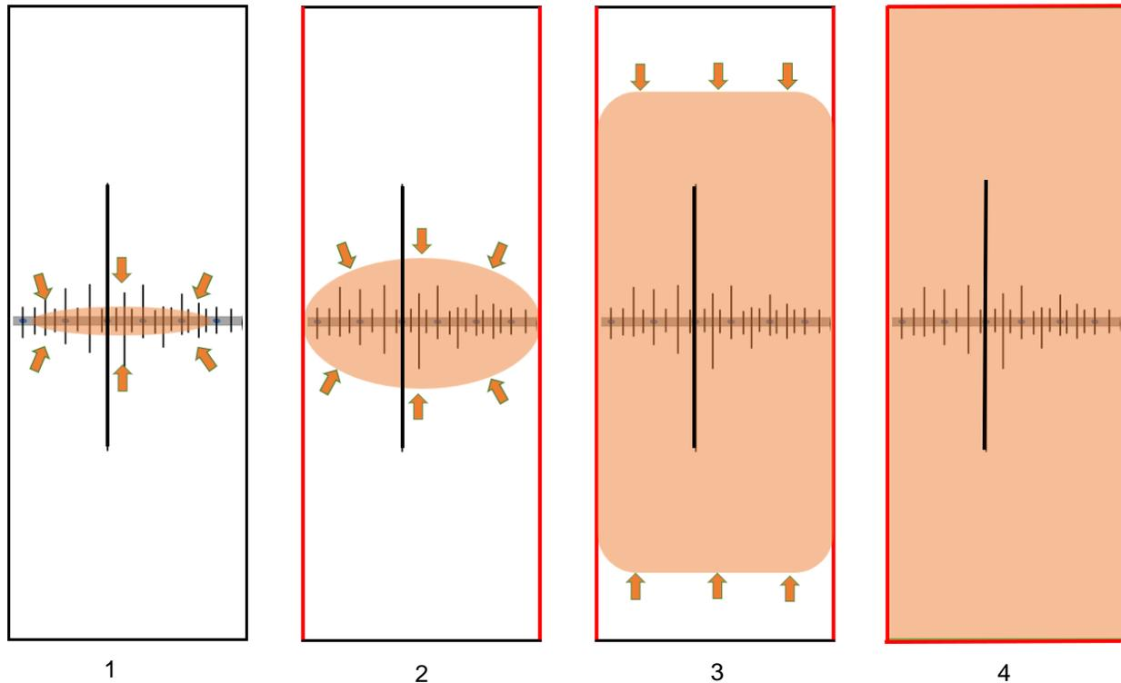
Figure 5 - Simplified model with flow regime sequence (1) Early intra stage fracture interference (2) Boundary between stages/dominant fractures (3) Linear channel flow (4) Fully bounded flow
