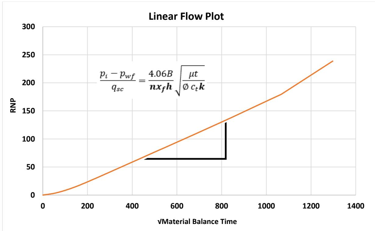
Figure 2 - Linear flow plot and equation for calculating fracture half length, number of stages and permeability (Olivier Houze, 2021). P is pressure in psi (subscript “i” is for initial and “wf” is for flowing pressure),  $q_{sc}$  is the rate in bbl./day, B is the formation volume factor (RB/STB),  $\mu$  is viscosity (cp), t is time (hours),  $\phi$  is porosity and  $c_t$  is the total compressibility (1/psi)
