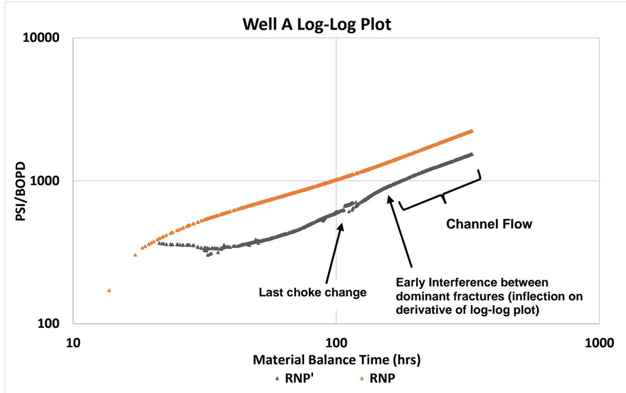
Figure 8 - The Log-Log Plot of initial production data for Well A shows an inflection on the derivative indicative of interference between stages / dominant fractures. This can only be seen with accurate hourly rate and pressure measurements.
