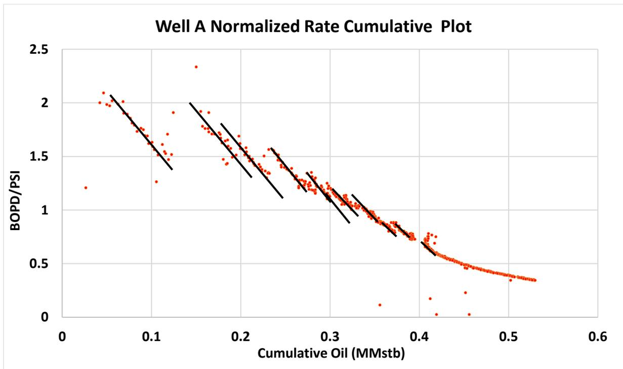
Figure 7 - Transients associated with each choke change in Well A are visible with good data quality
