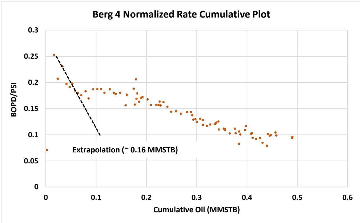
Figure 26 – Extrapolation to determine the volume at first boundary for Berg 4 data (~ 0.16 MMSTB). In contrast with Figure 7 transients associated with choke changes are not visible
