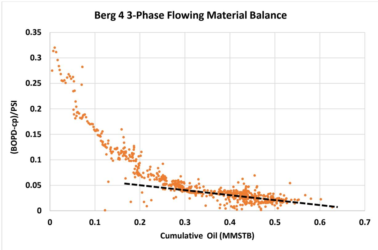
Figure 30 - A slope to the data 2.5 years indicating a volume of 0.64 MMSTB
