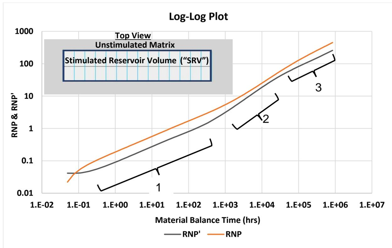
Figure 1 - Expected flow regimes for SRV bounded wells: 1. Linear flow into fractures 2. SRV Bounded Flow 3. Linear flow into SRV
