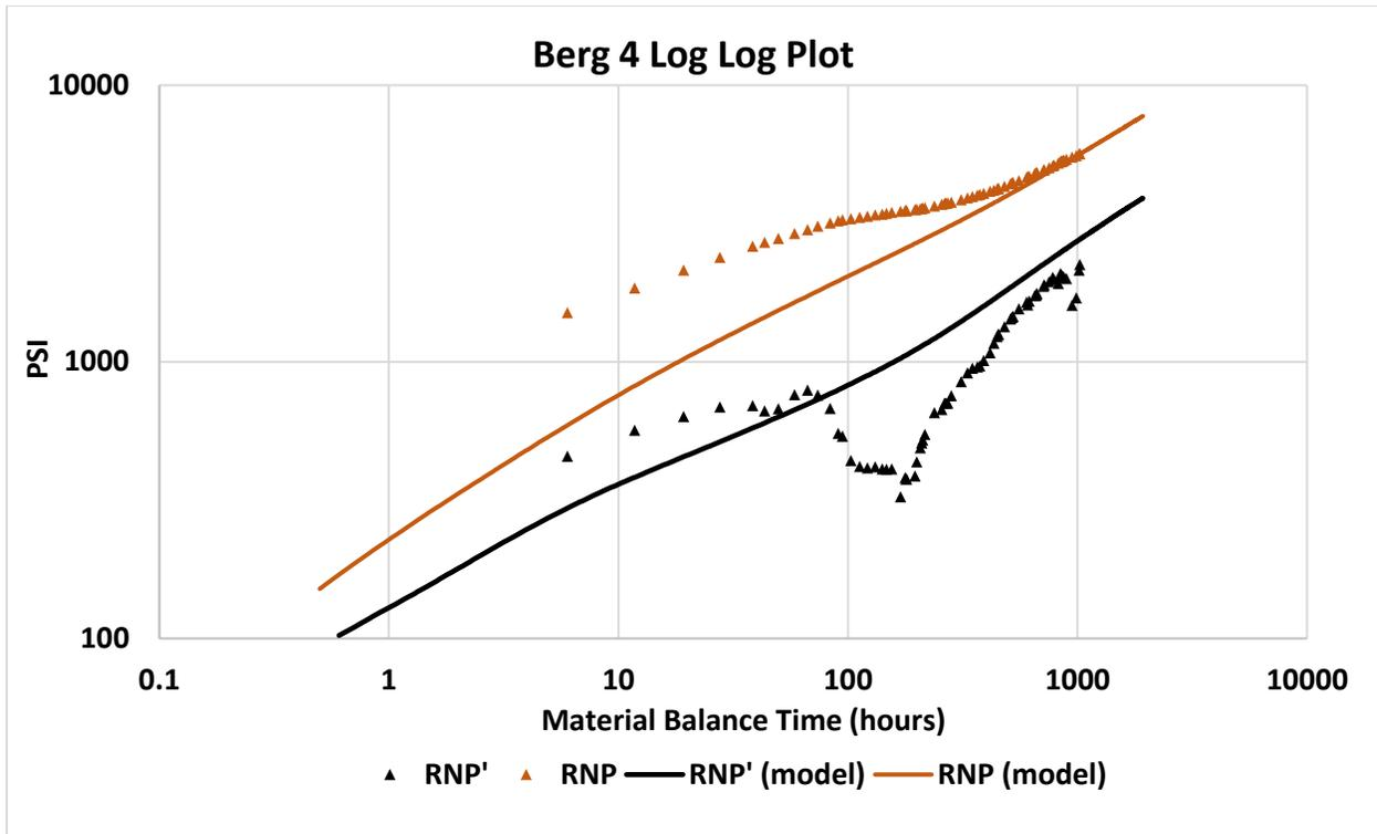
Figure 27 - Log-Log plot of model match to initial production data
