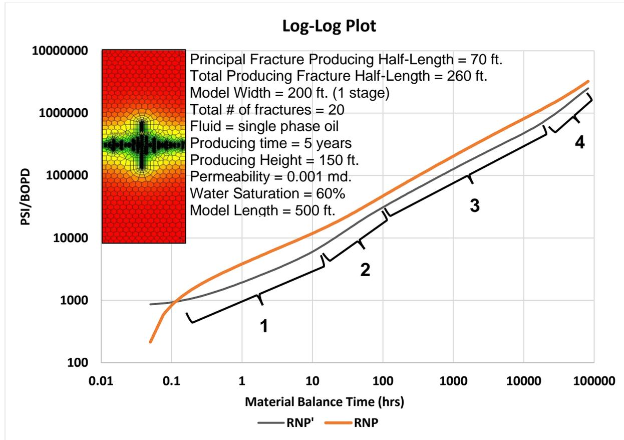
Figure 4 - Log-Log plot showing the model inputs and flow regime sequence for a single stage (1) Early linear / interstage fracture interference (2) Boundary between stages / dominant fractures (3) Linear channel flow (4) SRV or Boundary between wells
