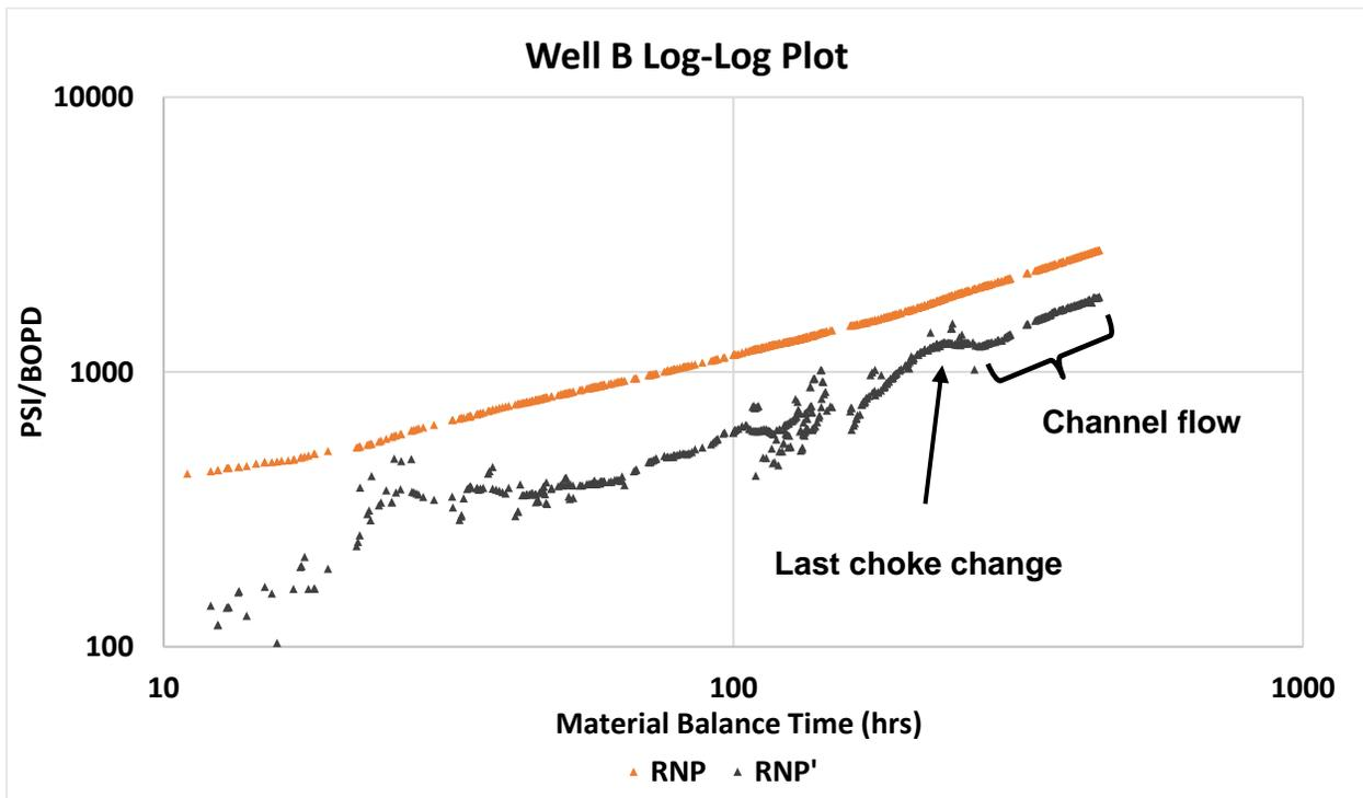
Figure 10 - Log-Log Plot for horizontal Eagle Ford well that shows how rate errors masks the inflection on the derivative indicative of the interference between dominant fractures.
