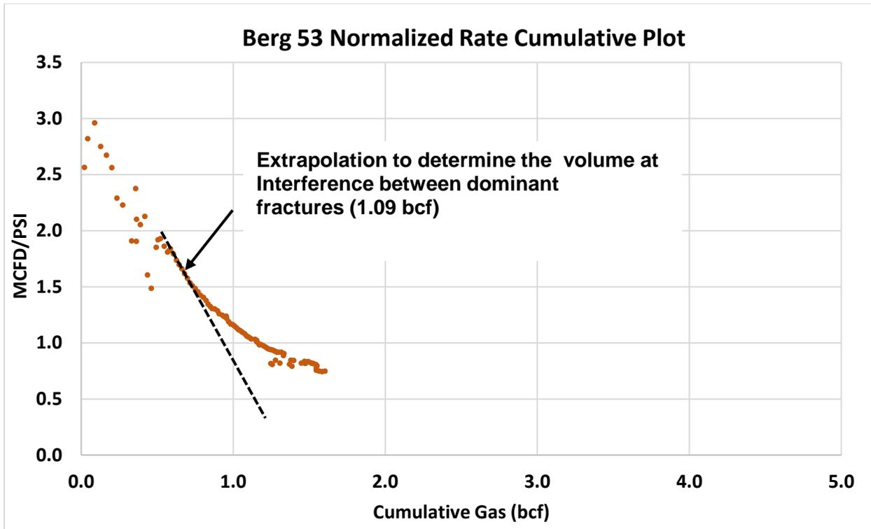
Figure 17 - Extrapolation for volume between dominant fracture / stages with daily data. In contrast with Figure 7 transients for choke changes are not visible
