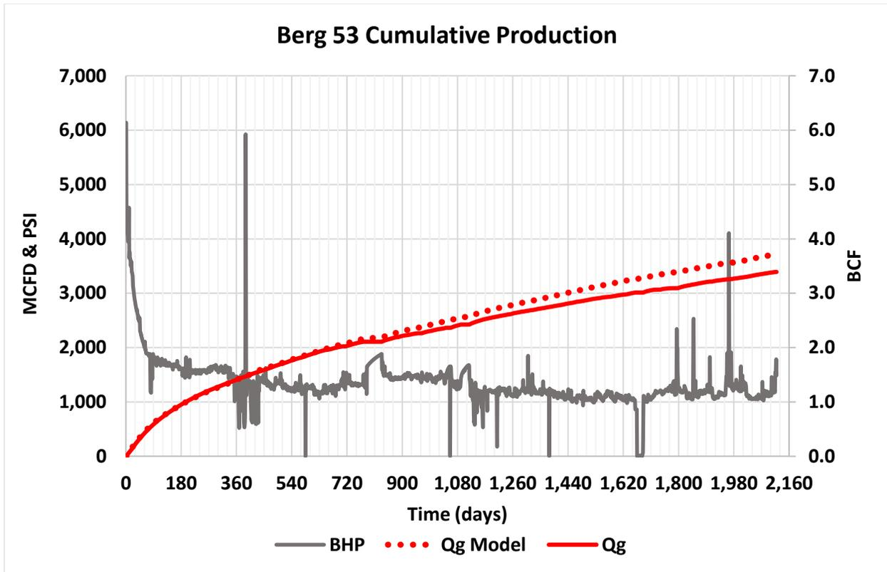
Figure 21 - Match using parameters determined from initial production data assuming each fracture drains a 8:1 channel.
