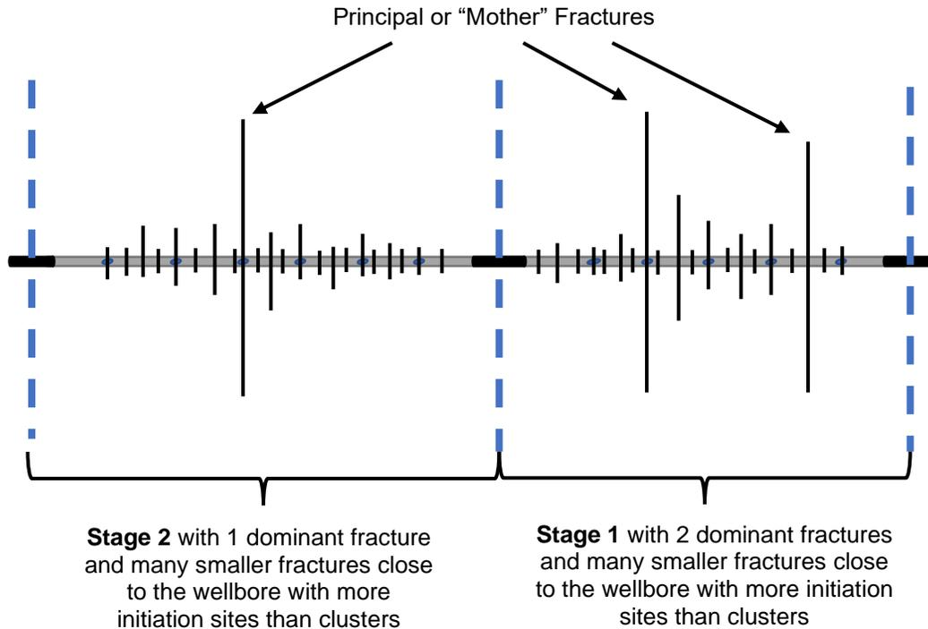
Figure 3 - Interpretation of basic fracture distribution and geometry from hydraulic fracturing test sites
