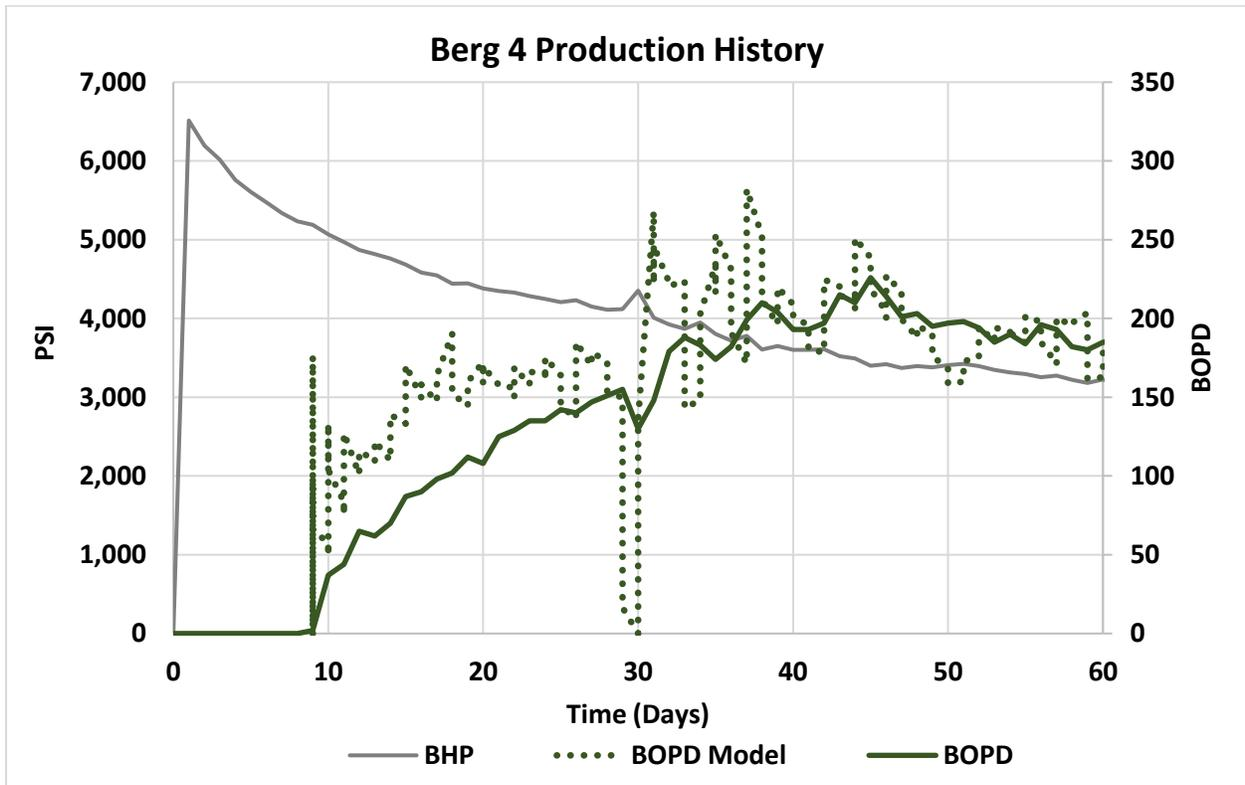
Figure 28 - Model match to first 2 months of data using the fracture half-length and permeability determined using initial production data
