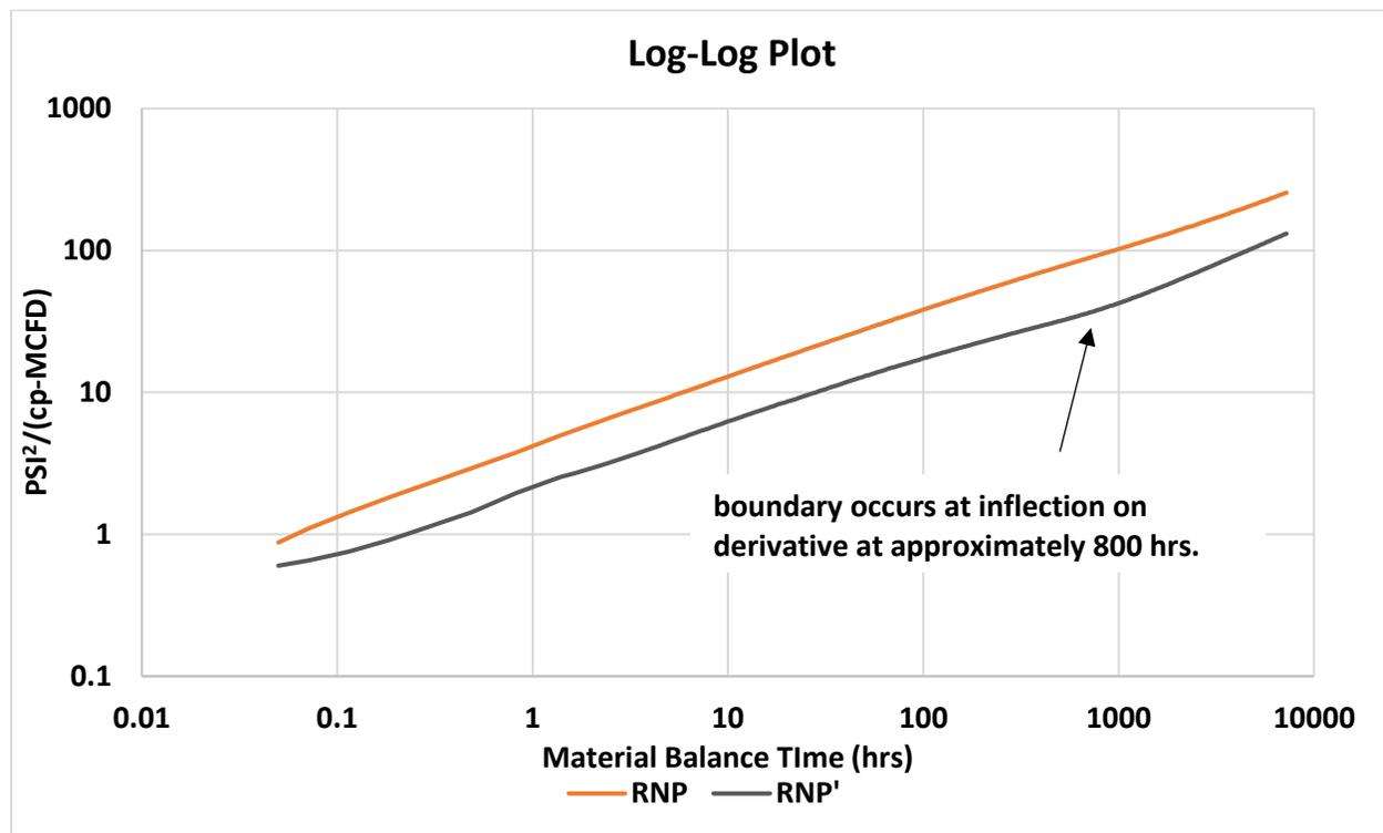
Figure 11 - Log-Log plot for single phase gas model showing early interference
