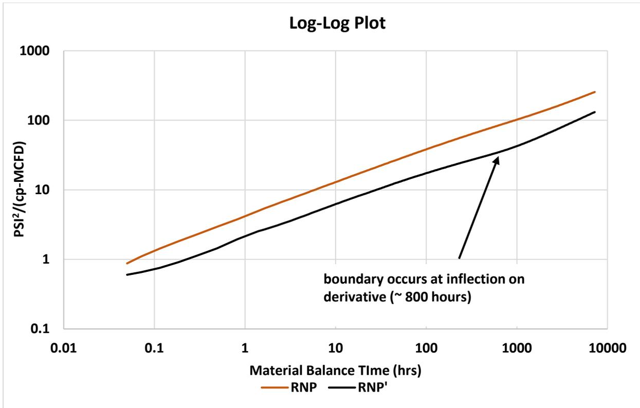
Figure 14 - Flow Regime Analysis showing interference at 800 hours
