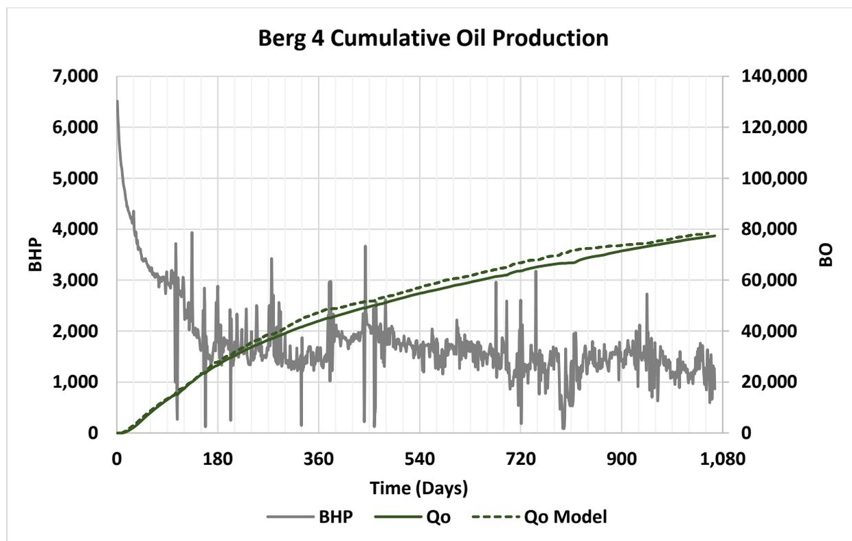
Figure 32 - Log-Log plot and cumulative production plot showing the model match constrained by the contacted volume in Figure 30
