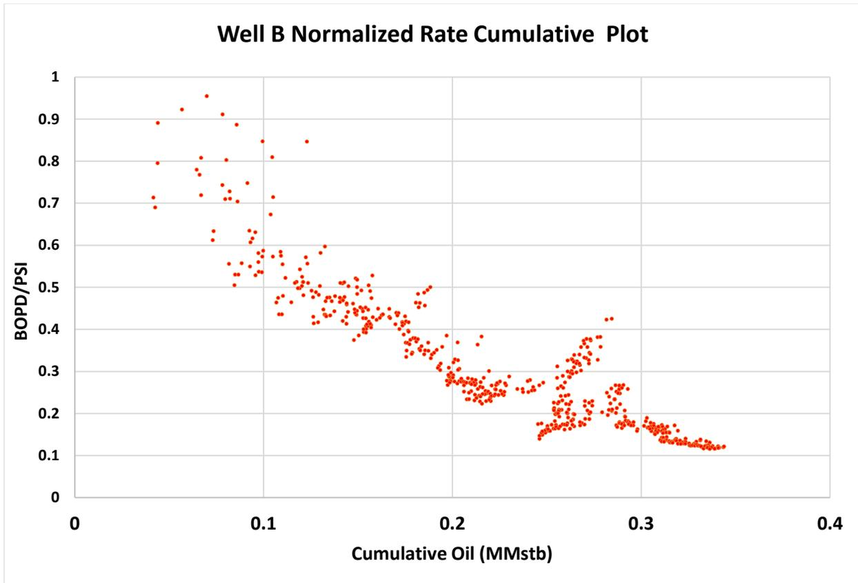
Figure 9 - Individual transients associated with each choke change cannot be seen because data quality is poor
