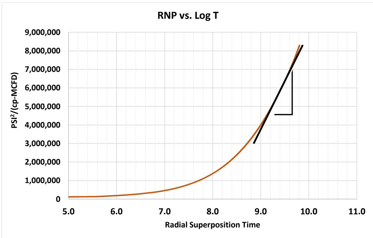
Figure 13 - Slope (black line) to the data from which permeability and fracture half-length are calculated. The solution assumes radial flow as defined by Lee, et al. (2003)
