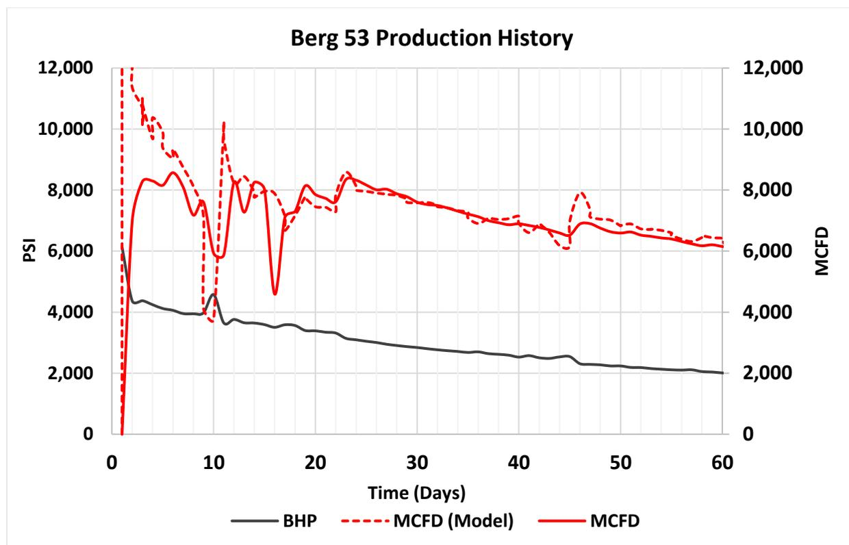
Figure 20 - Model match production history to first 2 months of data with the fracture half-length and permeability determined from initial production.
