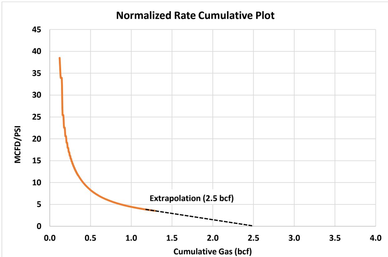
Figure 15 - Volume at interference for multi-stage example
